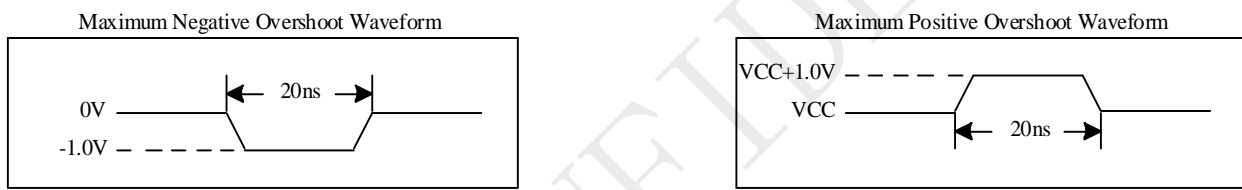
Figure 5-2 Input Test Waveforms and Measurement Level
