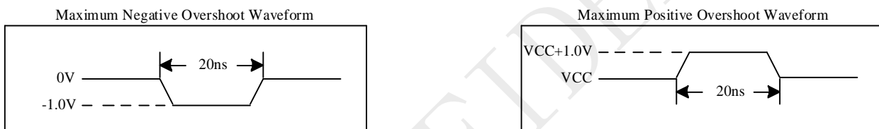
Figure 5-2 Input Test Waveforms and Measurement Level
