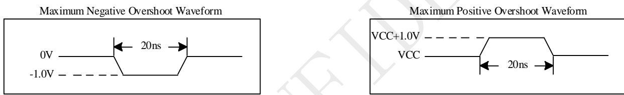
Figure 5-2 Input Test Waveforms and Measurement Level
