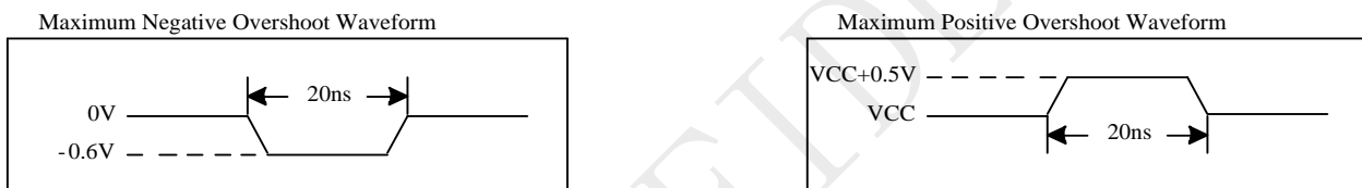
Figure 5-1 Maximum Overshoot Waveform
