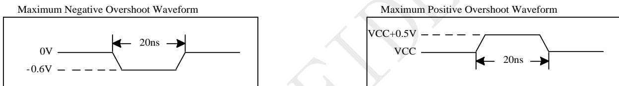
Figure 5-1 Maximum Overshoot Waveform
