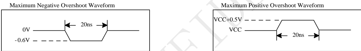
Figure 5-1 Maximum Overshoot Waveform
