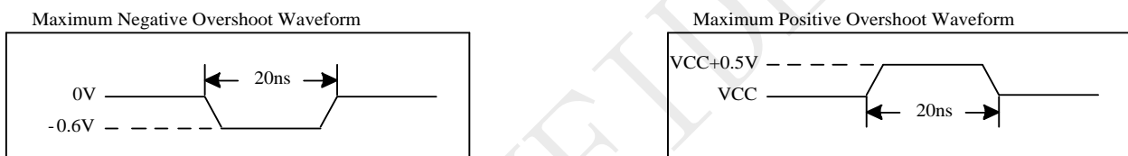
Figure 5-1 Maximum Overshoot Waveform
