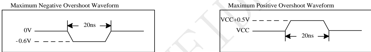
Figure 5-1 Maximum Overshoot Waveform
