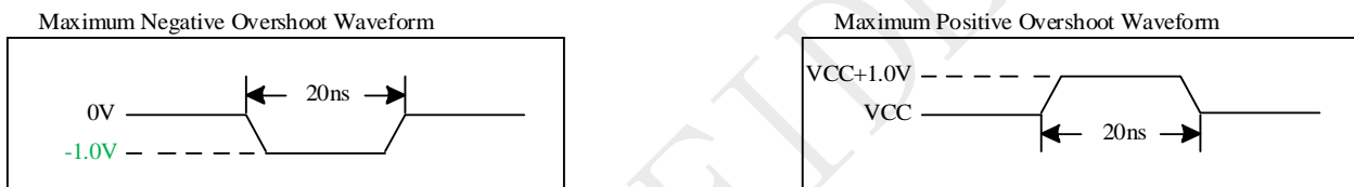
Figure 5-1 Maximum Overshoot Waveform
