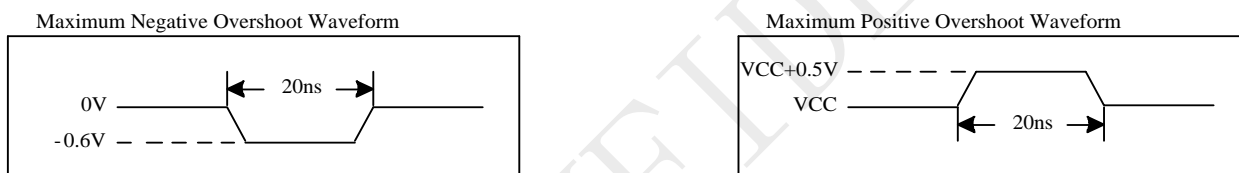
Figure 5-1 Maximum Overshoot Waveform
