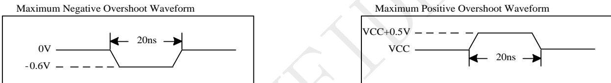
Figure 5-1 Maximum Overshoot Waveform
