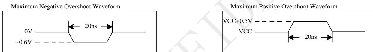
Figure 5-1 Maximum Overshoot Waveform
